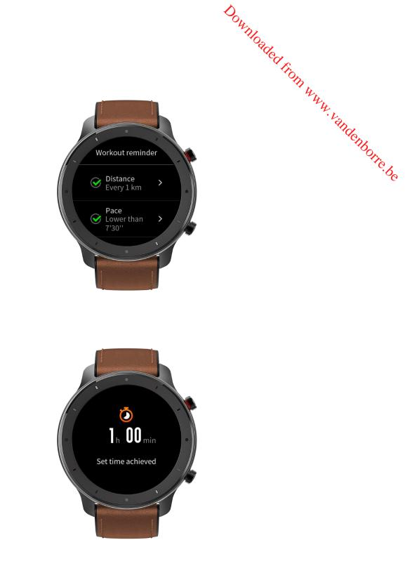
The workout reminder supports five types: distance, pace, safe heart rate, heart rate zone, and pace With a reminder set, the watch will vibrate to remind you as long as the set value is reached during workouts.
