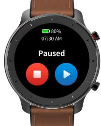
Tapping the right button can cancel the pause and resume the workout. Tapping the left button can end the current workout and save the workout performance.
