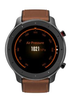
Sliding up on the air pressure page can enable you to enter the altitude page. The altitude requires double calibration of watch barometer and GPS. If you want more accurate altitude data, try to get the satellite positioning in an open area as soon as possible.
